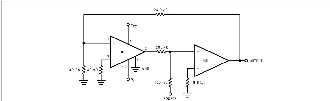
(1) DC Electrical Test; Refer to Test Circuit #1.
