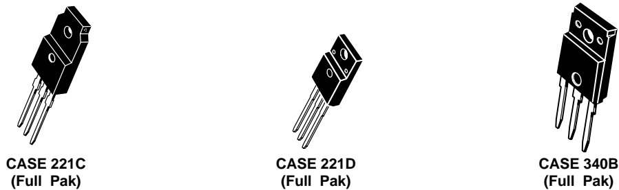
Figure 5–13. Plastic Body Mounted Packages
